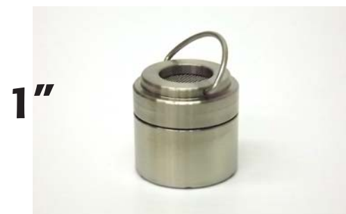
1" Large Capacity Holder (Material: SS316) - Cat# 8771A Interior 0.7" Ht x 1.0" I.D. (17.8 mm Ht x 25.4 mm I.D.) Exterior 1.05" Ht x 1.20" O.D. (26.7 mm Ht x 30.5 mm O.D.) Mesh Material: SS 316 / Mesh Size: 35x35 / Opening: 0.017" (0.43mm)
