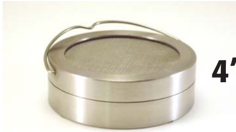
4" Large Capacity Holder (Material: SS316) - Cat# 8771D Interior 0.7" Ht x 4.0" I.D. (17.8 mm Ht x 101.6 mm I.D.) Exterior 1.05" Ht x 4.4" O.D. (26.7 mm Ht x 111.8 mm O.D.) Mesh Material: SS 316 / Mesh Size: 35x35 / Opening: 0.017" (0.43mm)
